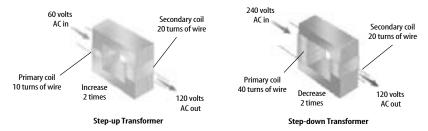
**Step-Up Transformer** A step-up transformer increases voltage so that the output voltage is greater than the input voltage. The secondary coil then has more turns than the primary coil. In the first figure, an input voltage of 60 volts in the primary coil provides an output voltage of 120 volts in the secondary coil. The secondary coil has twice as many turns as the primary coil has. Therefore, the output voltage is twice as large as the input voltage.
